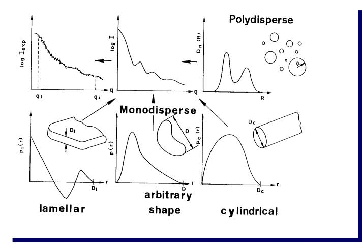
The IFT technique can also be applied to data from cylindrical or lamellar particles as well as to polydisperse systems
