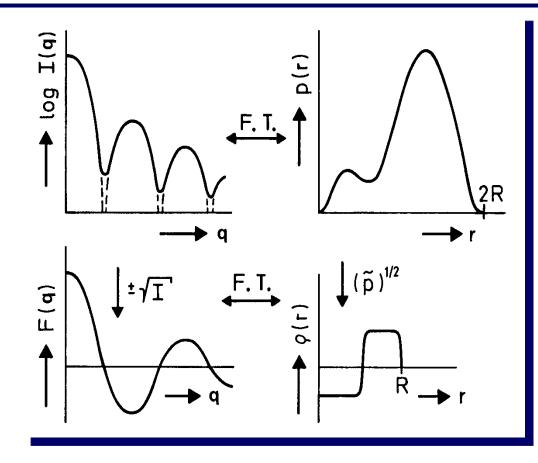
Deconvolution of the PDDF p(r) into the radial density  $\Delta \rho(r)$  is possible for:
