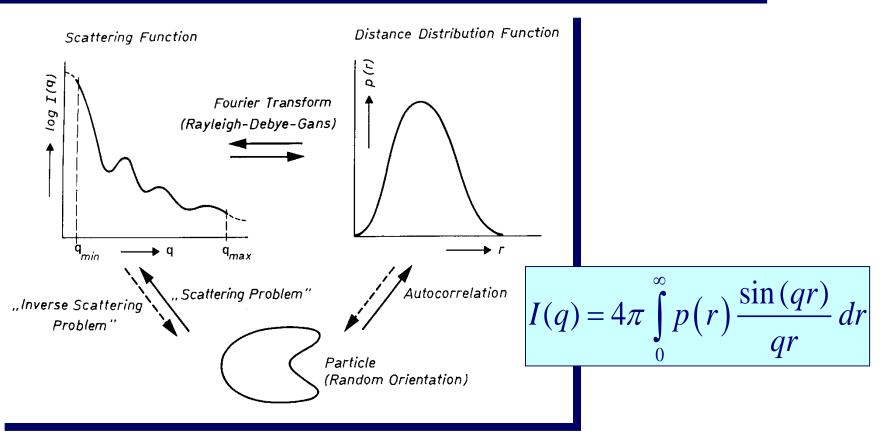
For the solution of the inverse Problem it is essential to be able to calculate the PDDF form the experimental scattering curve with minimum termination effect without model assumptions.
