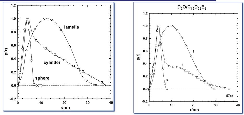
Pair distance distribution functions p(r) for the binary mixture  $D_2O/C_{12}D_{25}E_5$ at 5 °C (circles), 32 °C (squares), and 70 °C (triangles). These functions are obtained by indirect Fourier transformation of the SANS spectra.
